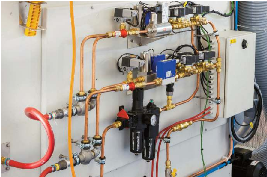
Gas mass flow control, ignition and flame detection system mounted on the Gas Diverter plate (cover not shown)
