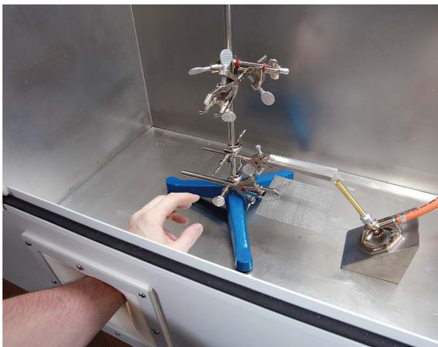
Easy entry to the chamber via one of the two access ports
