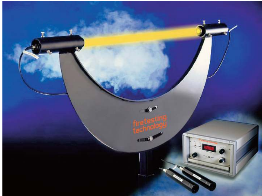
White light smoke measurement system
