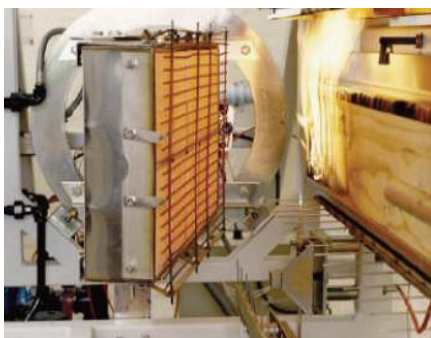
Panel box assembly with reverberatory screen as mounted in equipment test frame.
