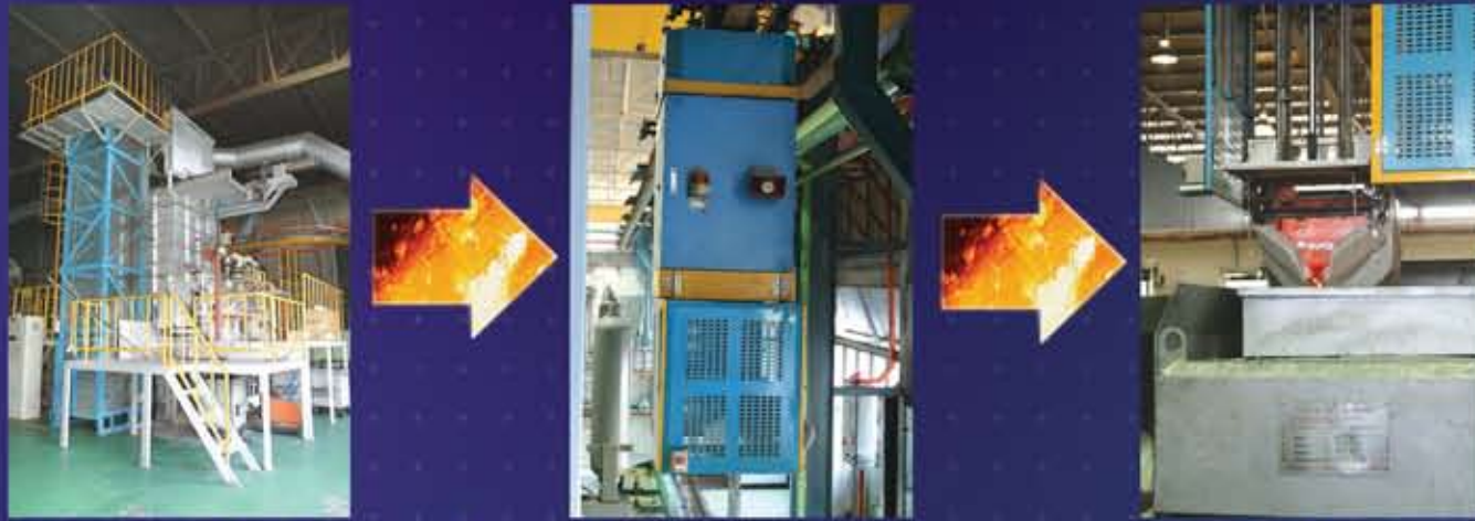
Central Aluminum Melting Furnace Automated Molten Aluminium Transporter Electric Holding Furnace Capacity ranging between 12,000 kg to 48,000 kg molten aluminium per day
