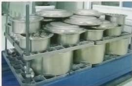
氮化后工件外观 The parts after Nitrided
