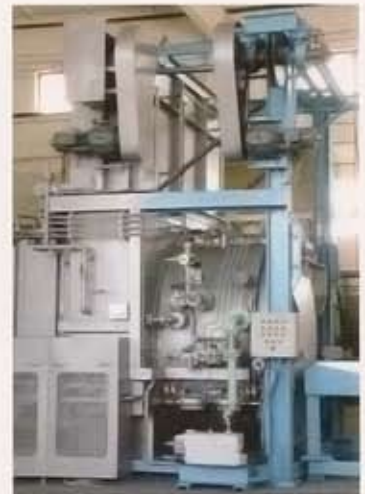
真空锁气室 (用于等温退火线) Vacuum lock chamber (for Isothermal annealing)
