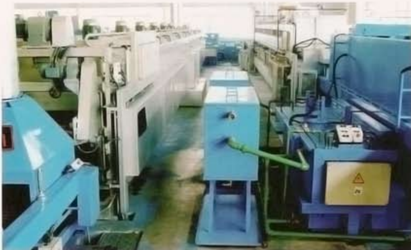
真空锁气室 (用于等温退火线) Vacuum lock chamber (for Isothermal annealing)
