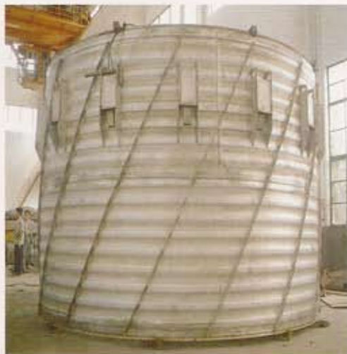
制作中的特大型井式炉耐热钢波纹马弗及相配套的耐热钢波纹导风筒 Heat resistant steel Retort and Heat resistant steel cylinder are in building
