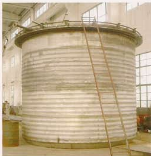
制作中的特大型井式炉耐热钢波纹马弗及相配套的耐热钢波纹导风筒 Heat resistant steel Retort and Heat resistant steel cylinder are in building
